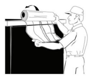
1. From the endwall of the container, place the roll in the center of the container rim. Unroll 1 foot of the liner so that it hangs down the outside of the container. While holding on to the end of the liner, shove the roll over the rim, allowing it to unroll across the bottom of the container to the opposite end.
