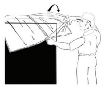
2. Unfold the liner, ensuring that the center slit remains centered in the container. DO NOT TEAR THE END SEAM OF THE LINER. From the endwall, pull the top layer of the liner toward you as shown. Fold it over one corner of the container and then over the other corner.
